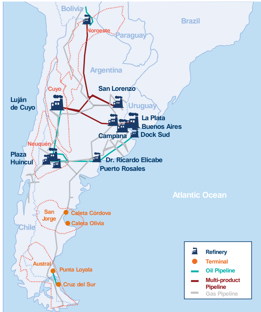
Figure 24 – Map of Oil, Gas, and Multipurpose Pipelines in Argentina
